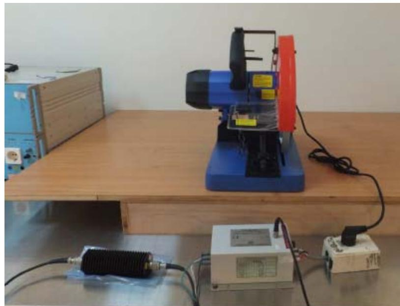
Figure 7 Conducted RF disturbances immunity test setup
