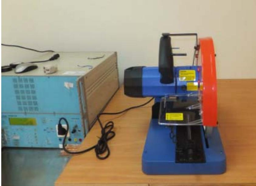
Figure 4 Harmonics & Flicker & Surge & DIPS test setup
