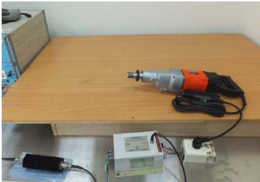
Figure 7 Conducted RF disturbances immunity test setup
