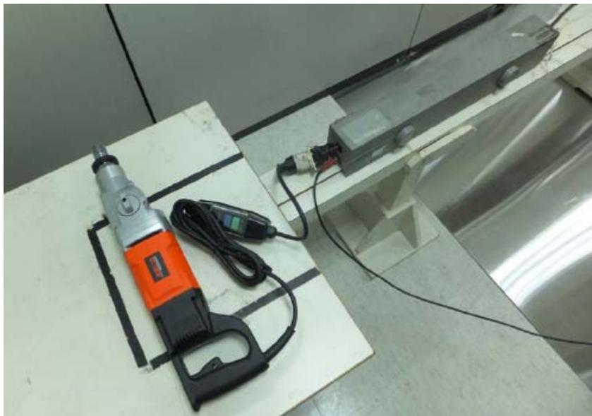
Figure 3 Disturbance power test setup
