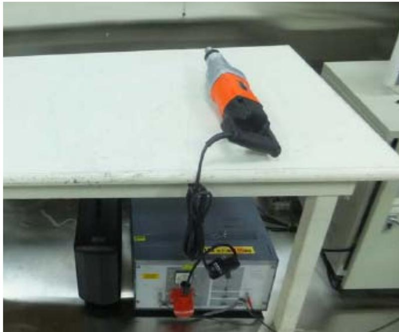
Figure 2 Conducted Emission test setup
