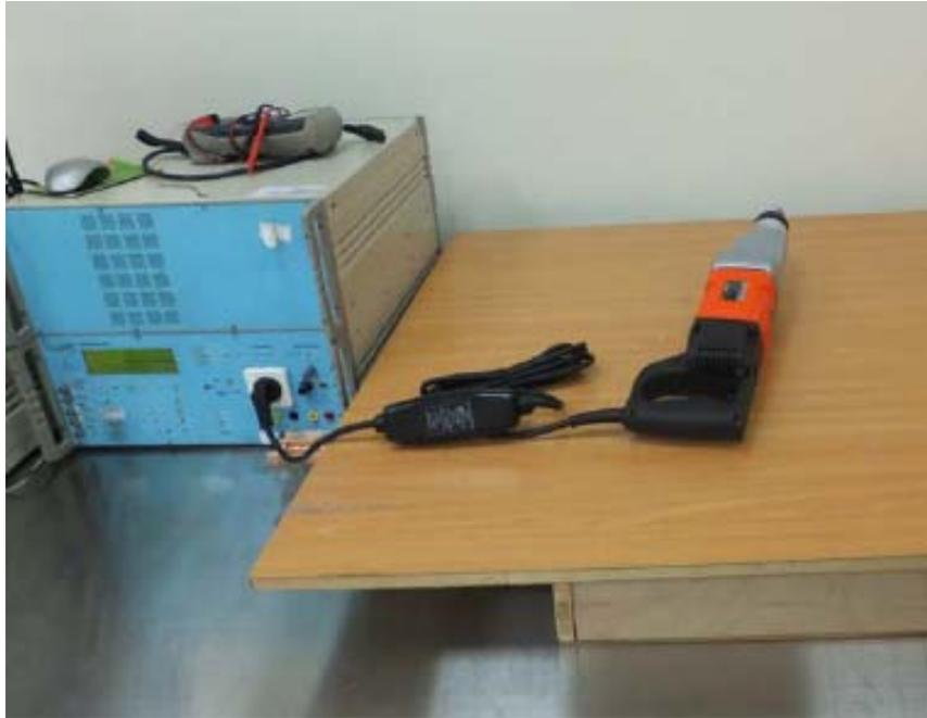
Figure 6 EFT test setup
