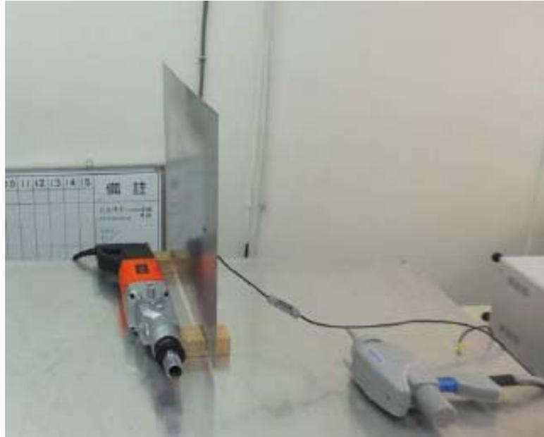
Figure 5 ESD test setup
