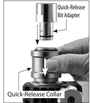
**CAUTION: Keep the surfaces of the Quick-Release Bit Adapter and the inside of the Quick-Release Collar assembly clean. Accumulated dust and slurry could cause them to become jammed together.**
