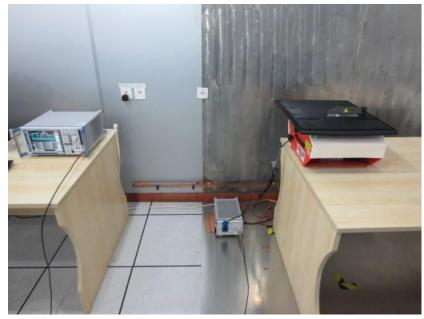
Figure 3 Conducted Emission test setup
