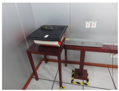
Figure 4 Disturbance power test setup
