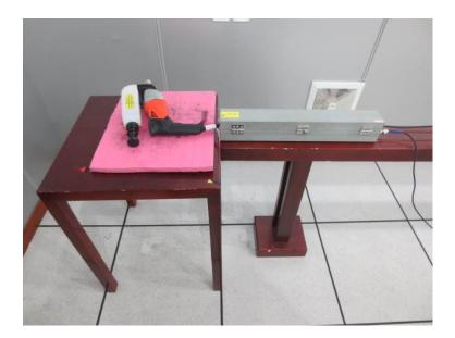
Figure 5 Disturbance power test setup
