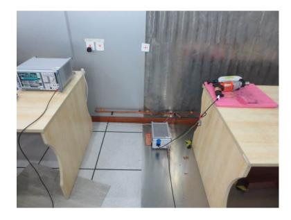
Figure 4 Conducted Emission test setup
