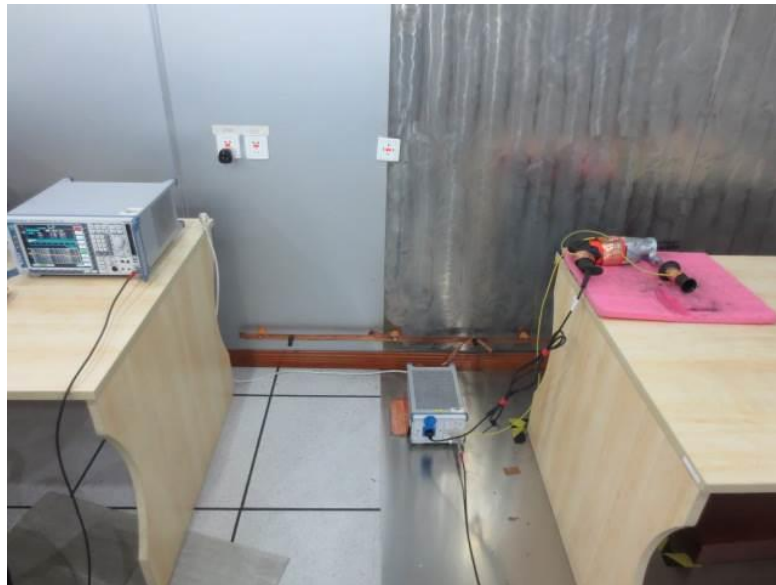
Figure 3 Conducted Emission test setup
