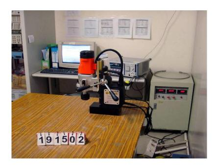
Figure 3 Conducted Emission test setup
