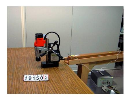
Figure 4 Disturbance power test setup
