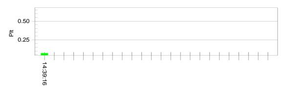
Parameter values recorded during the test:Vrms at the end of test (Volt):228.28Highest dt (%):0.21Time(mS) > dt:0.0Highest dc (%):0.00Highest dmax (%):0.19Highest Pst (10 min. period):0.160Highest Plt (2 hr. period):0.070
