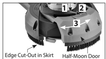
**NOTE: Keep the mechanism clean. Accumulated dust will make it difficult to open.**
