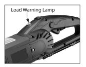
is exceeded and sustained for too long, the motor will shut down and the load warning lamp will glow solid red. In this case, the motor must be first shut off and then restarted.
