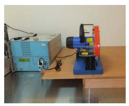
Figure 6 EFT test setup
