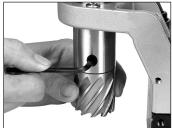
Ensure that the oil feed tap is on and coolant feeds properly by pushing the pilot pin. If it feeds too quickly or slowly, adjust the tap accordingly. Keep the tap closed when not in use.
