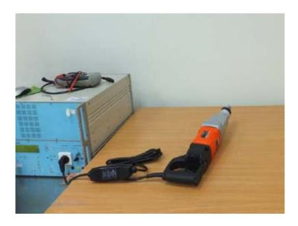
Figure 4 Harmonics & Flicker & Surge & DIPS test setup
