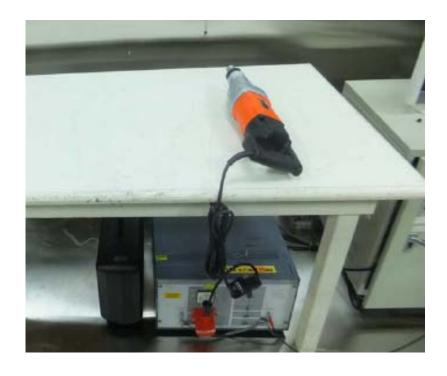
Figure 2 Conducted Emission test setup
