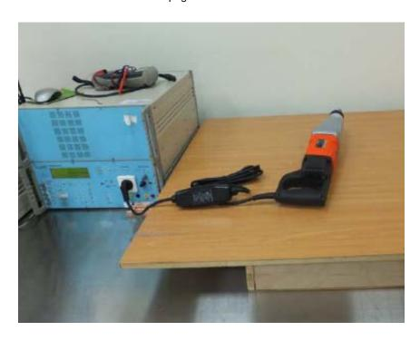
Figure 6 EFT test setup
