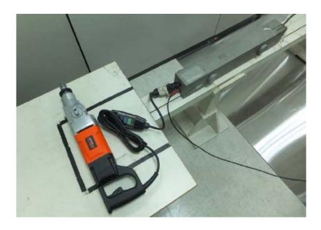
Figure 3 Disturbance power test setup
