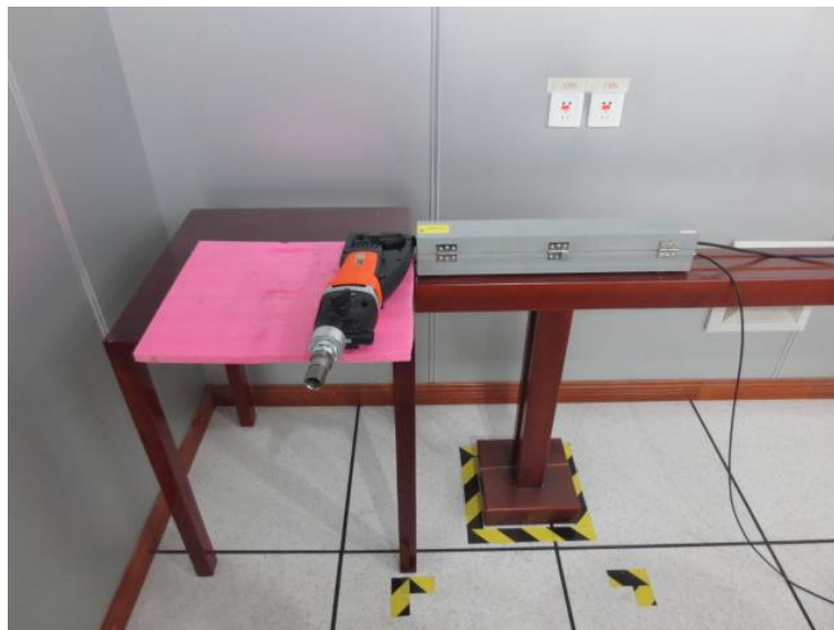
Figure 4 Disturbance power test setup
