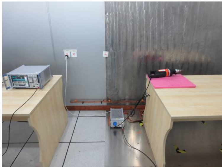
Figure 3 Conducted Emission test setup
