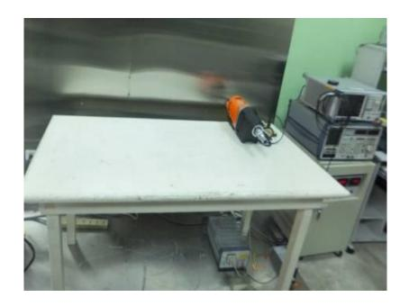
Figure 3 Conducted Emission test setup
