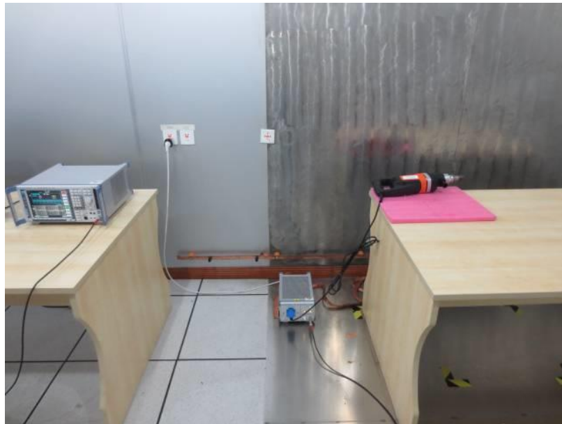
Figure 3 Conducted Emission test setup
