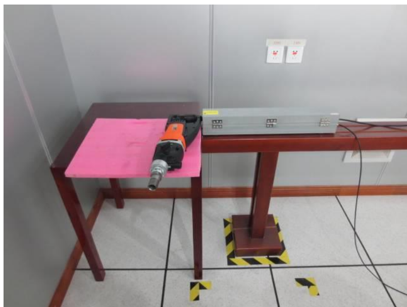
Figure 4 Disturbance power test setup
