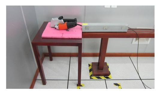
Figure 4 Disturbance power test setup
