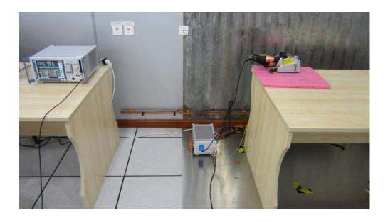
Figure 3 Conducted Emission test setup
