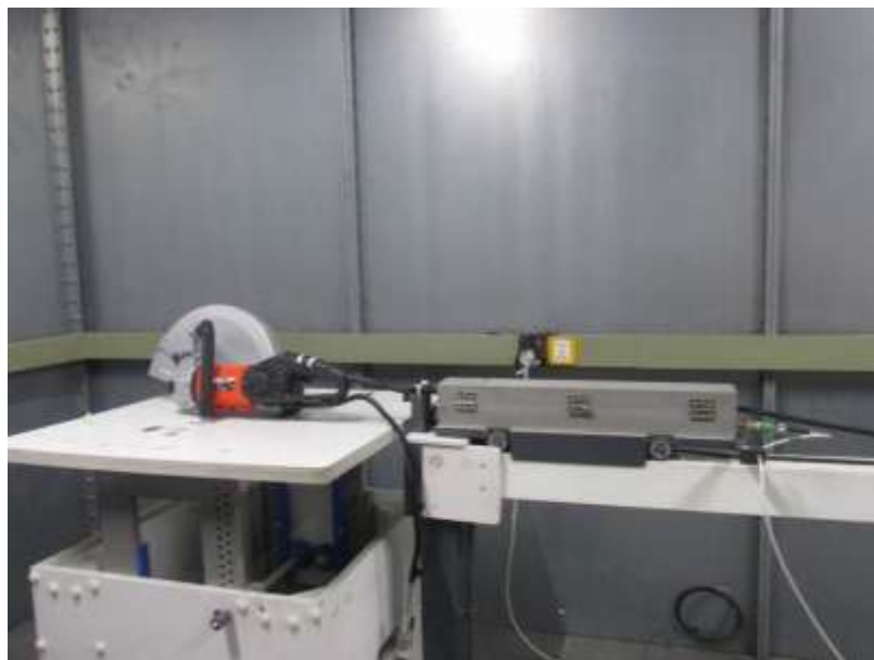
Figure 4 Disturbance power test setup
