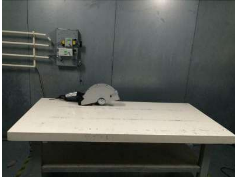
Figure 3 Conducted Emission test setup
