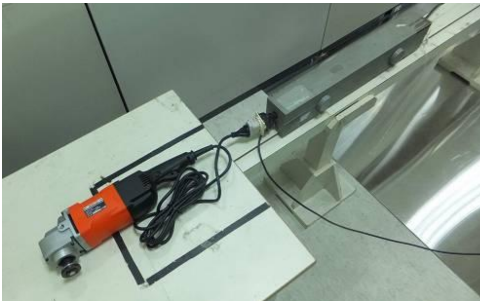
Figure 5 Disturbance power test setup
