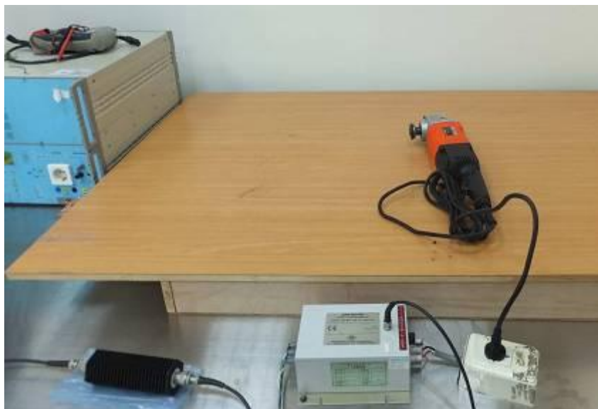
Figure 9 RF Conducted immunity test setup
