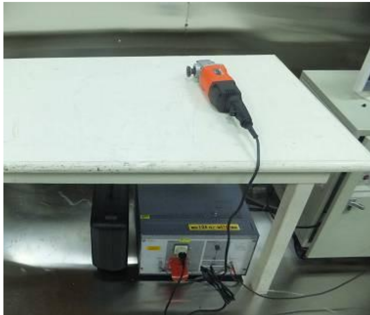
Figure 4 Conducted Emission test setup
