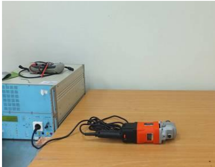
Figure 6 Harmonics & Flicker & Surge & DIPS test setup
