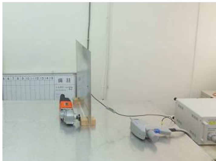
Figure 7 ESD test setup
