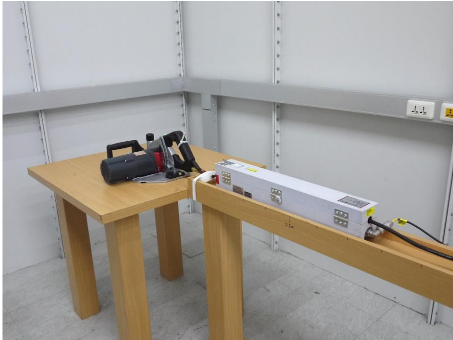
SCS8 (110-120 V) between EUT and protector
