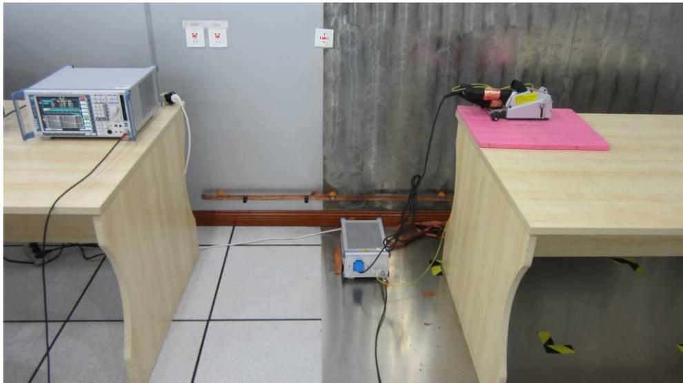
Figure 3 Conducted Emission test setup
