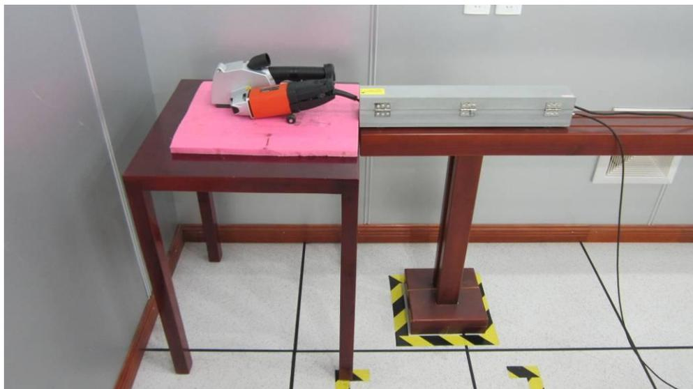
Figure 4 Disturbance power test setup
