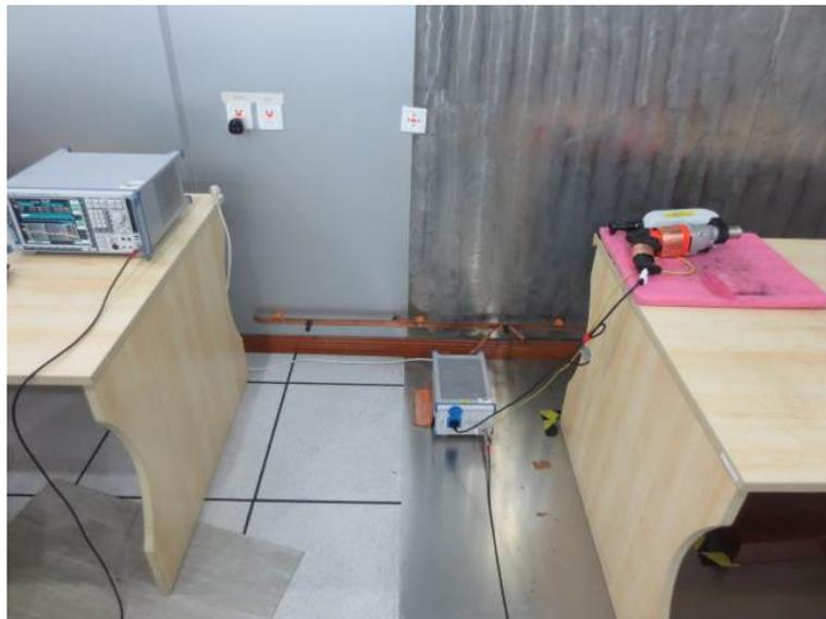
Figure 4 Conducted Emission test setup
