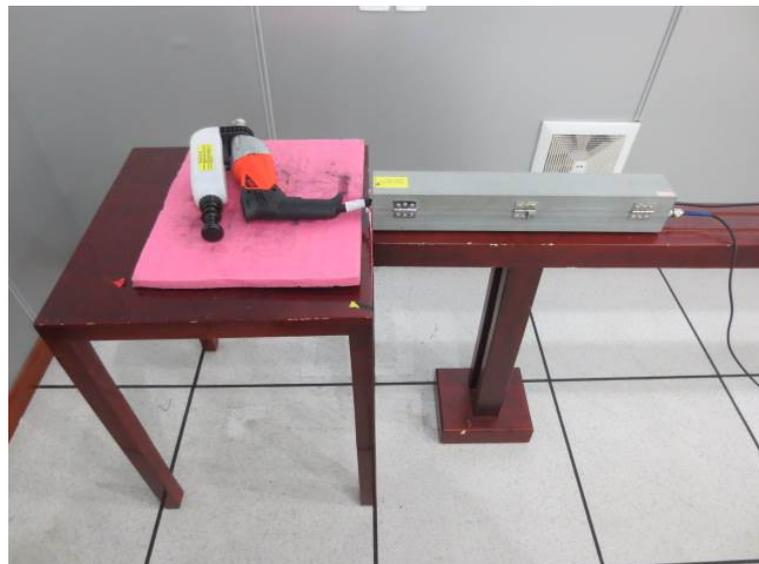
Figure 5 Disturbance power test setup
